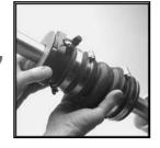
Carefully slide the assembly (hose end first) onto the shaft and onto the stern tube.
