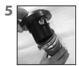
Place two hose clamps over each end of the articulating hose. Insert the C&MSeal TM into the hose as far as it will go. Tighten hose clamps around the C&MSeal TM.
